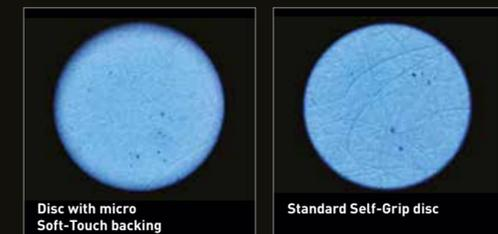
Discs with foam backing provide shallow scratches for quicker, easier polishing.
